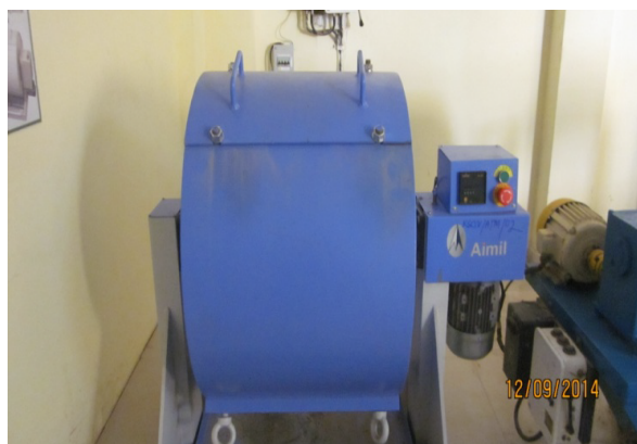
Figure 8: Los Angeles abrasion machine.
