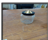
(b) Picnometer used for determination of water absorption
