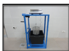
(a) Buoyancy balance use for specific gravity
