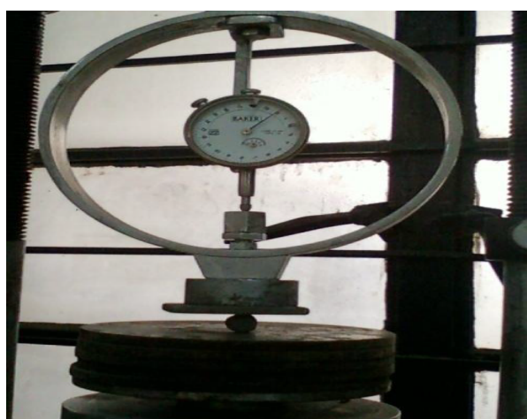
Figure 6: Testing setup for individual crushing strength of pellet.
