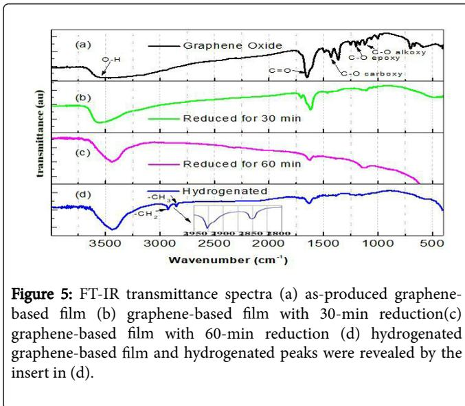
**Figure 5:** FT-IR transmittance spectra (a) as-produced graphene-based film (b) graphene-based film with 30-min reduction (c) graphene-based film with 60-min reduction (d) hydrogenated graphene-based film and hydrogenated peaks were revealed by the insert in (d).
