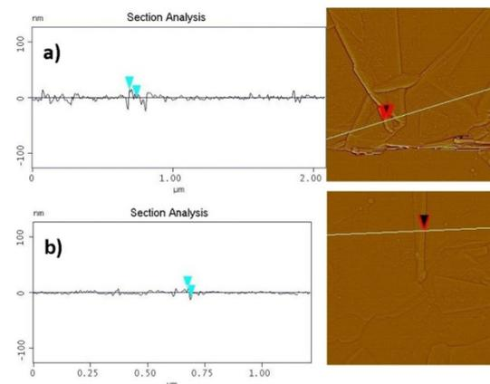
**Figure 4:** Atomic force microscopy (AFM) images (a) graphene-based film with 30-min reduction (b) hydrogenated graphene-based film.
