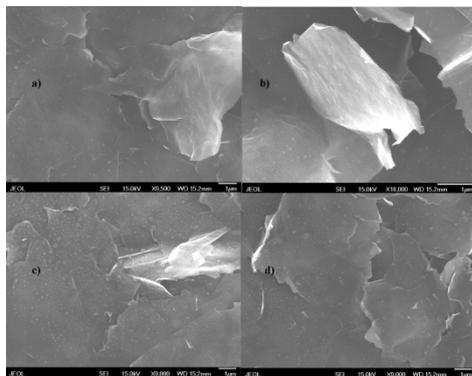
**Figure 2:** Scanning electron microscopy (SEM) images (a) as-produced graphene-based film; (b) graphene-based film with 30-min reduction (b) graphene-based film with 60-min reduction; c) hydrogenated graphene-based film.
