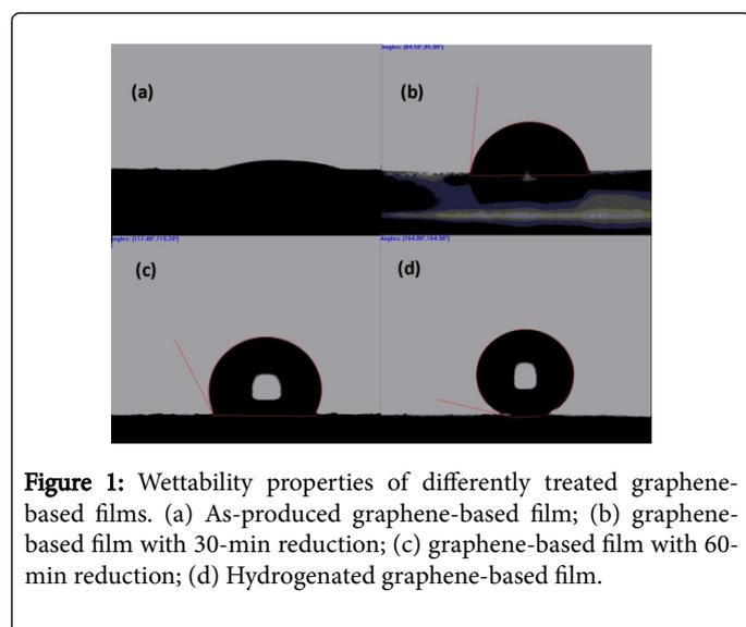
**Figure 1:** Wettability properties of differently treated graphene-based films. (a) As-produced graphene-based film; (b) graphene-based film with 30-min reduction; (c) graphene-based film with 60-min reduction; (d) Hydrogenated graphene-based film.
