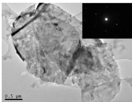
**Figure 3:** Transmission electron microscopy (TEM) image for hydrogenated graphene-based film; Insert is reciprocal lattice peaks obtained by 2D Fourier transform based on TEM image for hydrogenated graphene-based film.
