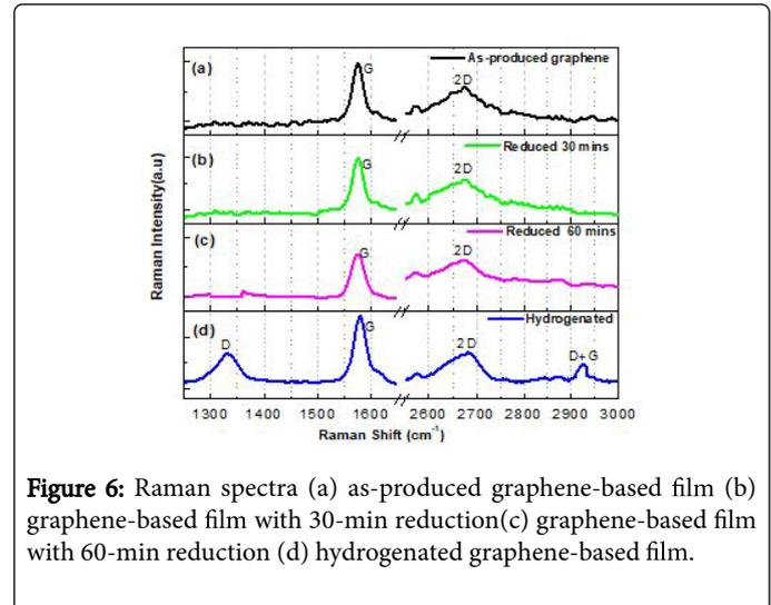
**Figure 6:** Raman spectra (a) as-produced graphene-based film (b) graphene-based film with 30-min reduction (c) graphene-based film with 60-min reduction (d) hydrogenated graphene-based film.
