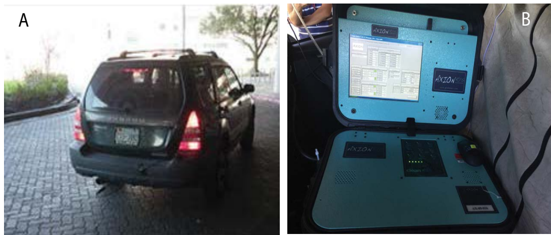
Figure 1: a) The test vehicle b) PEMS placed inside the test vehicle.
