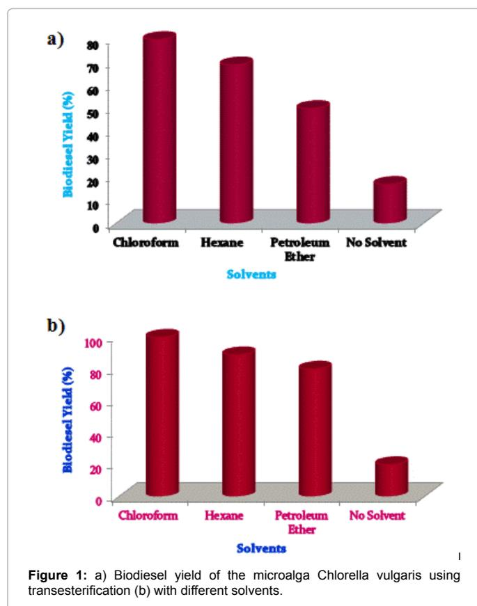
Figure 1: a) Biodiesel yield of the microalga *Chlorella vulgaris* using transesterification (b) with different solvents.
