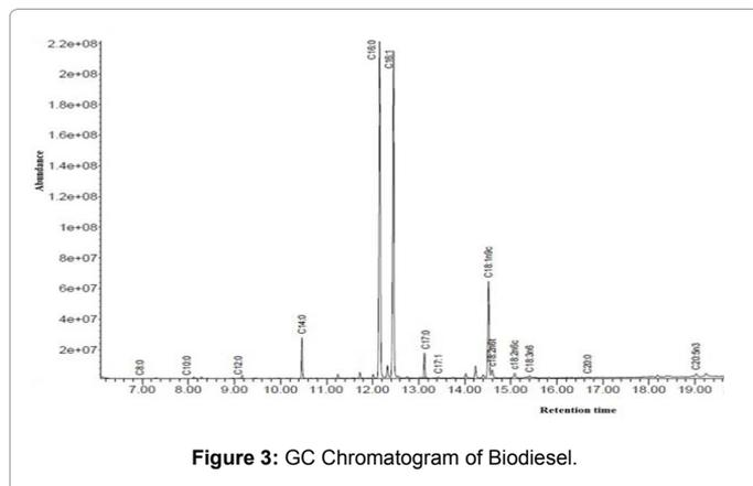
Figure 3: GC Chromatogram of Biodiesel.
