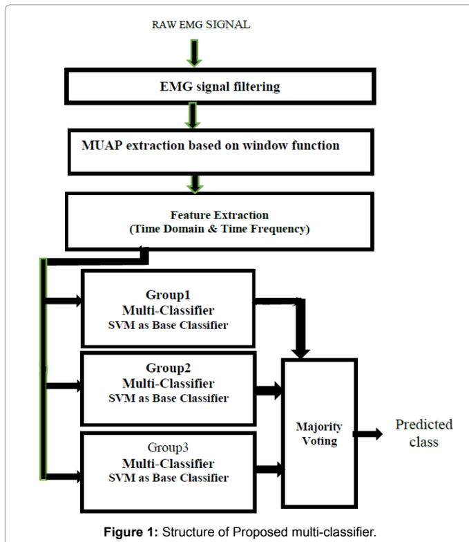
Figure 1: Structure of Proposed multi-classifier.
