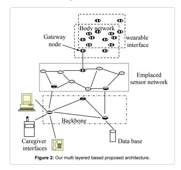
neighboring sensor nodes by a high-speed relay for efficient routing. The backbone may communicate wirelessly or may overlay onto an existing wired infrastructure. Nodes possess significant storage and computation capability, for query processing and location services. Yet, their number is minimized to reduce cost.
