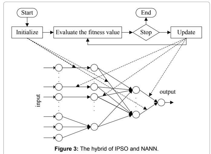
Figure 3: The hybrid of IPSO and NANN.
