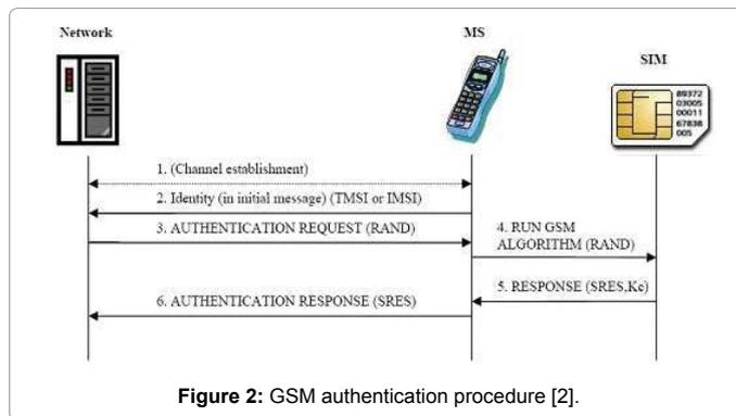
Figure 2: GSM authentication procedure [2].
