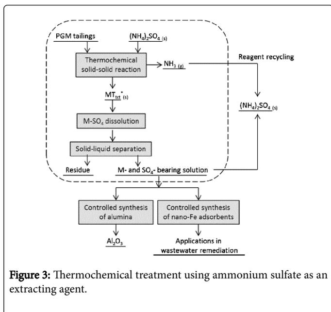
**Figure 3:** Thermochemical treatment using ammonium sulfate as an extracting agent.
