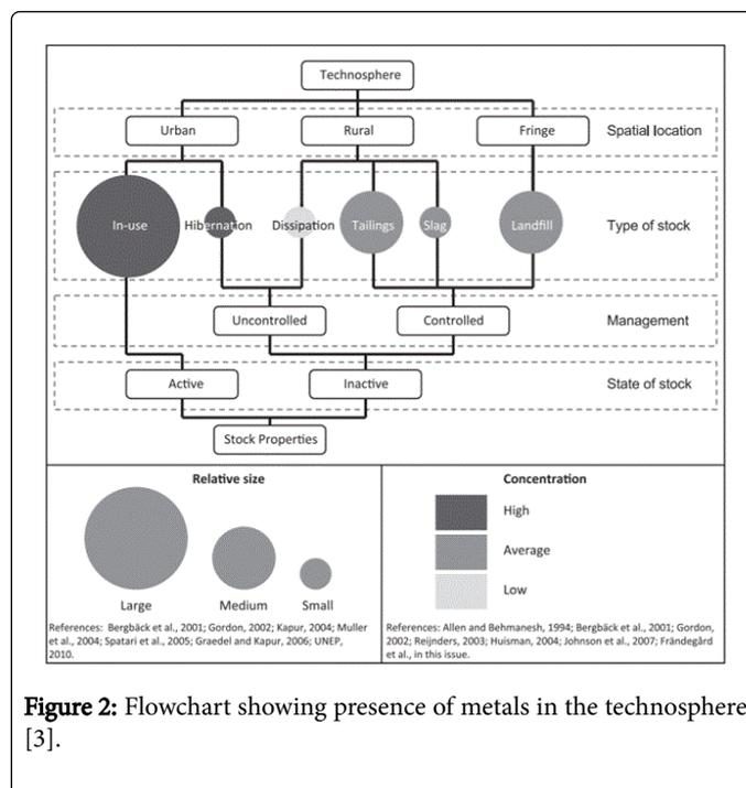
Figure 2: Flowchart showing presence of metals in the technosphere [3].
