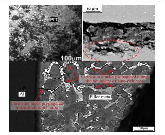
Figure 1: Common corrosion forms. (a) pitting corrosion, (b) intergranular corrosion, (c) stress corrosion.
