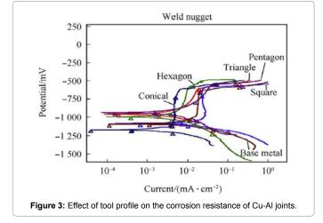
potential value of stir area processed changed with using different tools as shown in Figure 3 and Table 1 [24]
