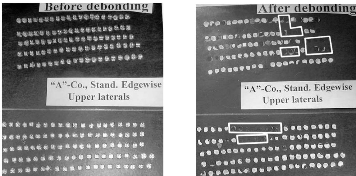
Figure 6. Tiles with new vs. OC-recycled brackets, before and after debonding
