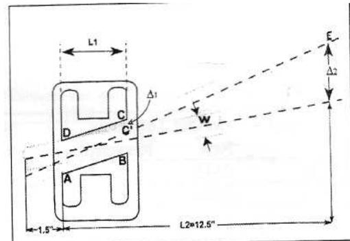
**Figure 4. Geometric representation of the arrangement in Figure 3**
