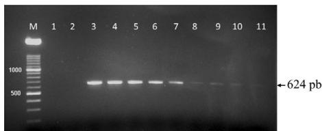
**Figure 5:** Detection of *PepMV* viral RNA in tomato extract. Two-fold serial dilution of extracted RNA were prepared in healthy plant extract and used as template in RT-PCR reactions. Target: *PepMV* RdRp gene (624 bp); Template quantity (25  $\mu$ l of reaction): (1) No template, (2) Healthy plant extract, (3) 140 ng, (4) 70 ng, (5) 35 ng, (6) 17.5 ng, (7) 8.75 ng, (8) 4.37 ng, (9) 2.19 ng, (10) 1.09 ng, (11) 0.55 ng.
