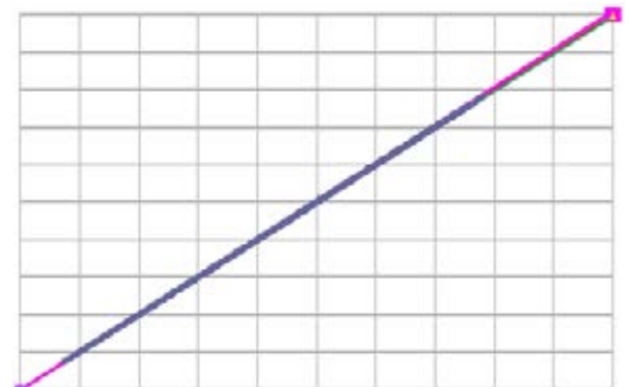
Figure 4: Comparison between values of Z_{crit} \cdot [\Phi_{\alpha}(Z)_{crit}]^{\frac{n-1}{n}} obtained by numerical code and the values calculated by equation (26).
