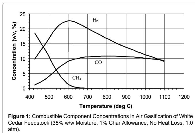
Figure 1: Combustible Component Concentrations in Air Gasification of White Cedar Feedstock (35% w/w Moisture, 1% Char Allowance, No Heat Loss, 1.0 atm).
