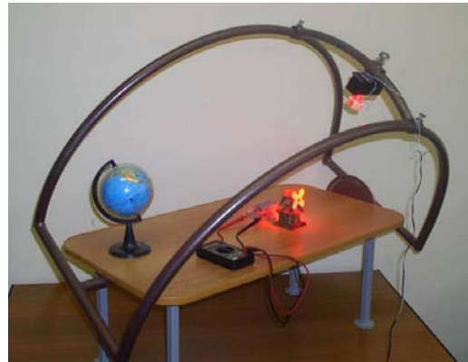
Fig. 17: Simulator of Sun's path on the sky for shadow analysis of solar buildings with small models (heliodon)
