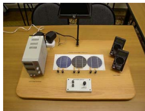
Fig. 12: Lab equipment for measuring characteristics of solar cells
