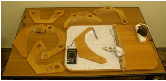
Fig. 13: Lab equipment for measuring characteristics of concentrators
