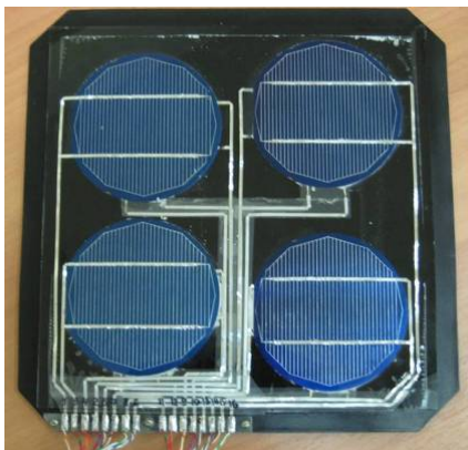
Fig. 16: PV/T receiving element of hybrid collector module
