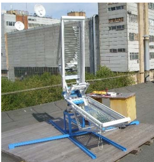
Fig. 10: Experimental concentrator for VEI PVT system
