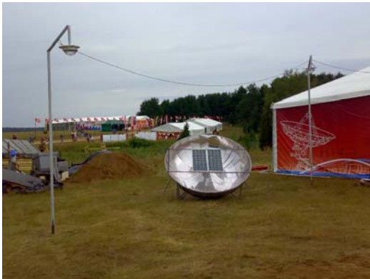
Fig. 2: Concentrator system is accumulating solar energy in camp for youth during daytime
