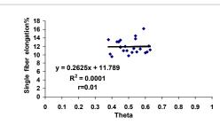
Figure 35: The relationship between single fiber elongation and theta.
