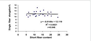
Figure 37: The relationship between single fiber elongation and SFC.
