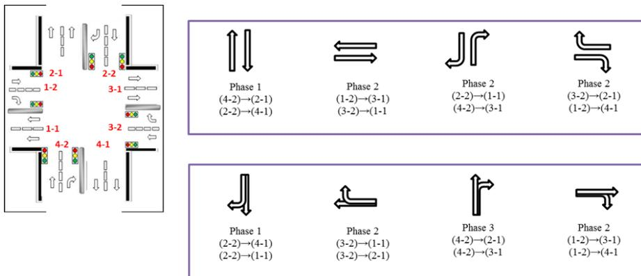
Figure 2: The typical intersection with Two Bunches of traffic Phases.
