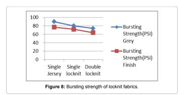
shows 74 and 64 PSI (Table 6 and Figure 8). It can be also discussed that locknit designs have more bursting strength than cross miss designs. It means that all knit course insertion in cross miss designs increases the bursting strength of the fabrics [14,15].
