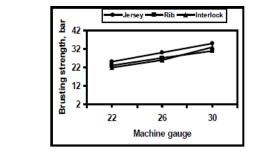
Figure 4: Effect of knitting machine gauge on knitted fabric Bursting strength for different knit structures.
