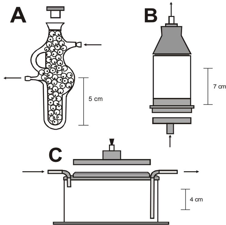
**Figure 2.** Water direction during the experiment in the respiration chamber.
