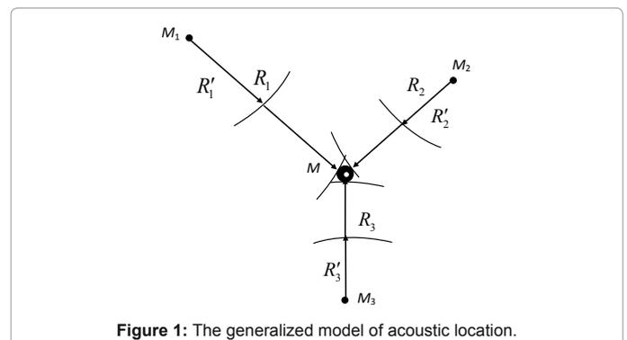
Figure 1: The generalized model of acoustic location.
