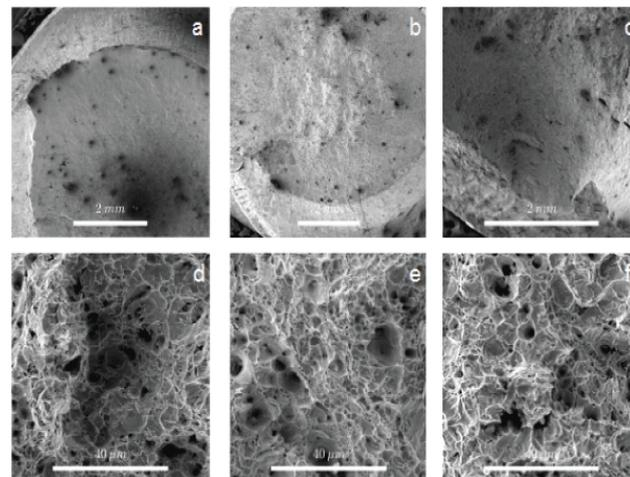
**Figure 4:** SEM micrographs of the fractured sections. (a-c) Low magnification images (32X) obtained from samples yellow, white and red respectively. (d-f) High magnification images (3000X) obtained from samples yellow, white and red respectively.
