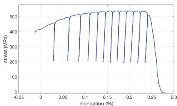
**Figure 3:** Representative low cycle force-controlled fatigue measurement performed on a steel reinforcing bar. In this particular example the number of cycles before the fracture was 12 and the final elongation 0.25%.
