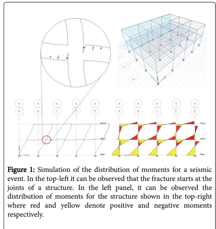
**Figure 1:** Simulation of the distribution of moments for a seismic event. In the top-left it can be observed that the fracture starts at the joints of a structure. In the left panel, it can be observed the distribution of moments for the structure shown in the top-right where red and yellow denote positive and negative moments respectively.
