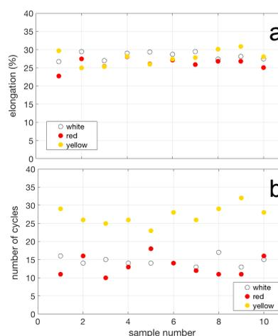
**Figure 5:** Results obtained from the low cycle force-controlled fatigue measurements of white, red and yellow rebars. (a) Elongation as a function of the number of tested samples. (b) Number of cycles before the fracture of the rebar as a function of the number of tested samples.
