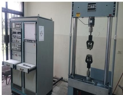
**Figure 2:** Universal testing machine MTS 810 utilized for low cycle force-controlled fatigue measurements.
