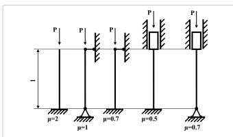
Figure 4: Shows several types of fixing rod and indicate the relevant values of the coefficient  $\mu$  - the so-called coefficient of length is given.
