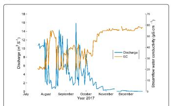
**Figure 3:** Discharge and electrical conductivity measurements at the Samendeni gauge station.
