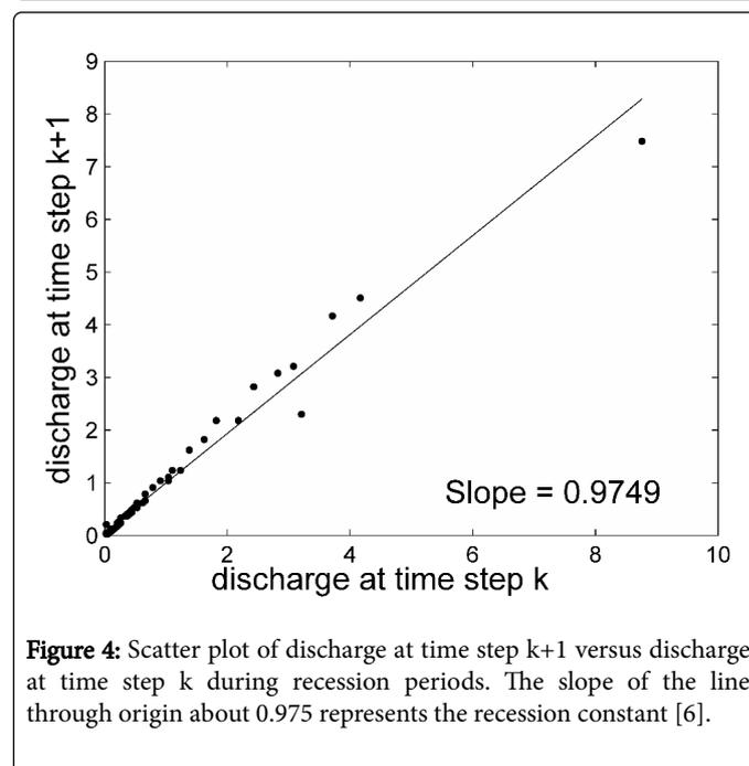
**Figure 4:** Scatter plot of discharge at time step  $k+1$  versus discharge at time step  $k$  during recession periods. The slope of the line through origin about 0.975 represents the recession constant [6].
