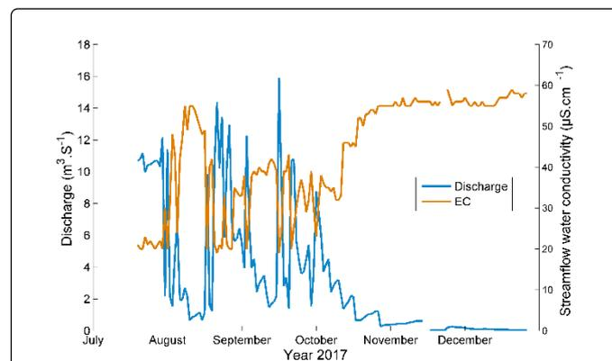
**Figure 3:** Discharge and electrical conductivity measurements at the Samendeni gauge station.
