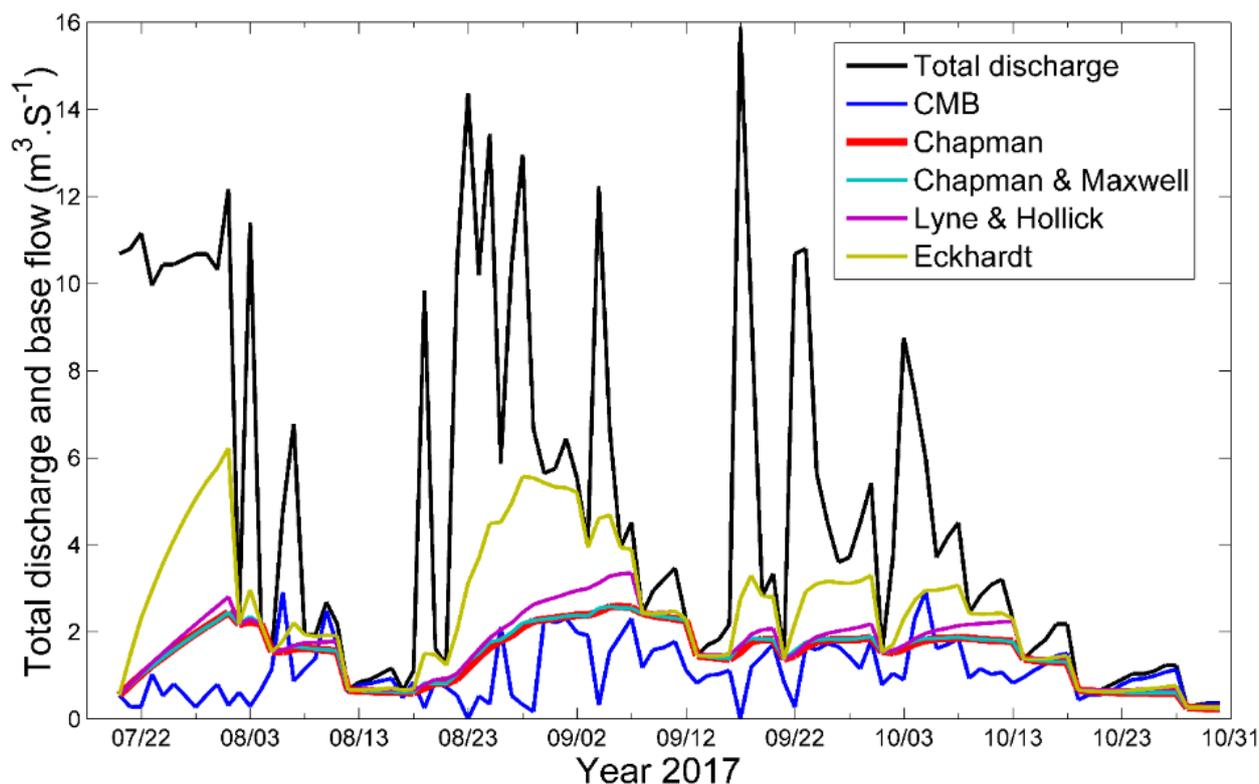
Figure 6: Temporal evolution of the total discharge and base flow from uncalibrated RDF methods and CMB method.
