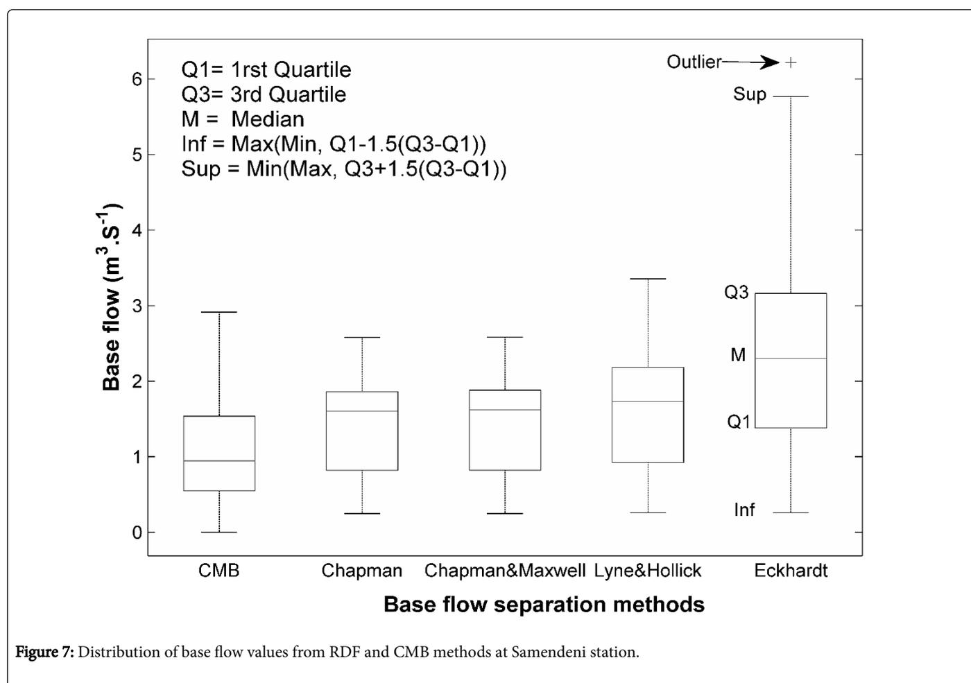
**Figure 7:** Distribution of base flow values from RDF and CMB methods at Samendeni station.
