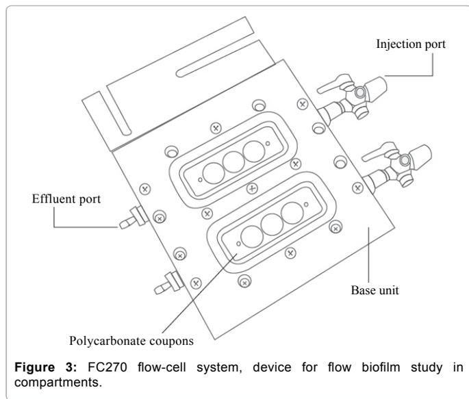
**Figure 3:** FC270 flow-cell system, device for flow biofilm study in compartments.
