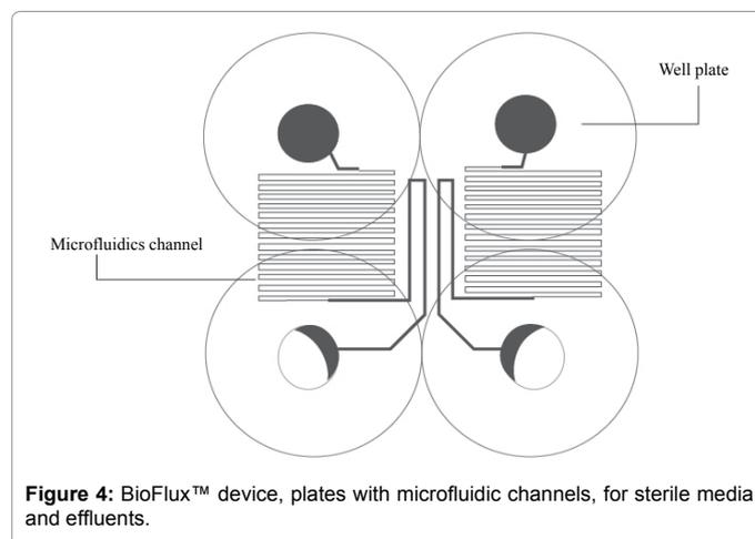
**Figure 4:** BioFlux™ device, plates with microfluidic channels, for sterile media and effluents.
