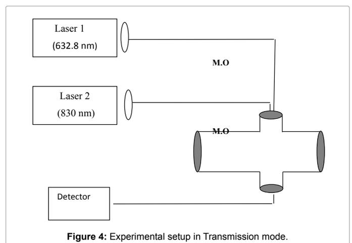
Figure 4: Experimental setup in Transmission mode.
