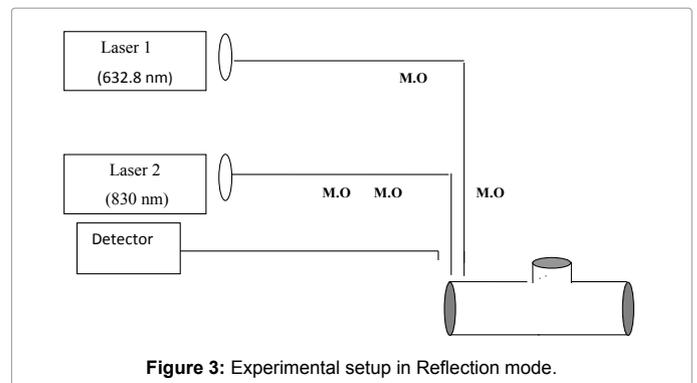
Figure 3: Experimental setup in Reflection mode.
