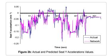
Seat X acceleration is inferior to Seat Y acceleration model in terms of catching the peaks and troughs of higher magnitude.
