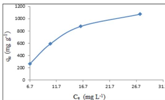
Figure 4: Plot of  $q_e$  vs.  $C_e$  for adsorption of Cr(VI) on to Fe<sub>3</sub>O<sub>4</sub> nanoparticles at pH 8.2, 0.01 g Fe<sub>3</sub>O<sub>4</sub>.
