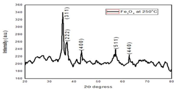
Figure 1: X-ray diffraction of magnetite nanoparticles at 250°C.
