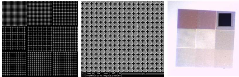
**Figure 3:** The patterns of the multispectral filters with 9 periodicities (left), the zoom in view of the pattern of periodicity of 450 nm (middle), the image under microscope (right).
