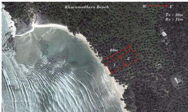
Figure 5: Loop configurations and direction of survey in the Khurumedhera Resistivity – salinity calibration.
