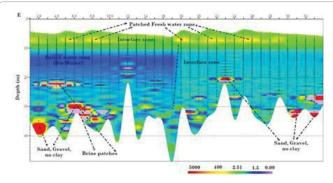
**Figure 8:** Fresh water aquifer in between the saline water aquifer in Khurumedhera Beach. The low TDEM resistivities between 11 to 17m depth are in agreement with the high groundwater salinity.
