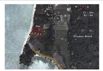
Figure 4: Loop configurations and direction of survey in the Wandoor.
