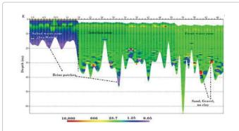
**Figure 7:** Fresh water aquifer in between the saline water aquifer in Wandoor Beach. The low TDEM resistivities between 7 to 18m depth are in agreement with the high groundwater salinity.
