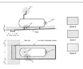
**Figure 3:** Zoning for Fuel tanks: a caption from standard IP15 showing the zones around a tank.
