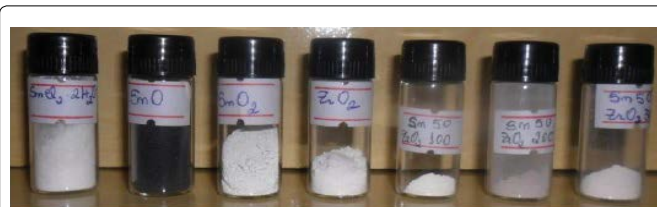
Figure 3: Samples of commercial and synthesized SnCl 2 /ZrO 2 supported catalysts a . a From left to right: tin(II) chloride dihydrate, tin(II) oxide, tin(IV) oxide, zirconium oxide, and composites SnCl 2 (50 wt. %)/ZrO 2 -100°C, SnCl 2 (50 wt. %)/ZrO 2 -200°C and SnCl 2 (50 wt. %)/ZrO 2 -300°C, respectively.
