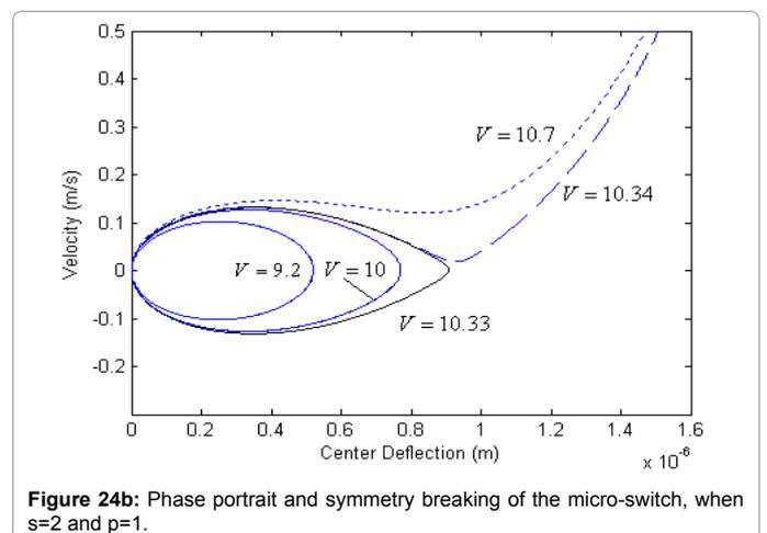
**Figure 24b:** Phase portrait and symmetry breaking of the micro-switch, when  $s=2$  and  $p=1$ .
