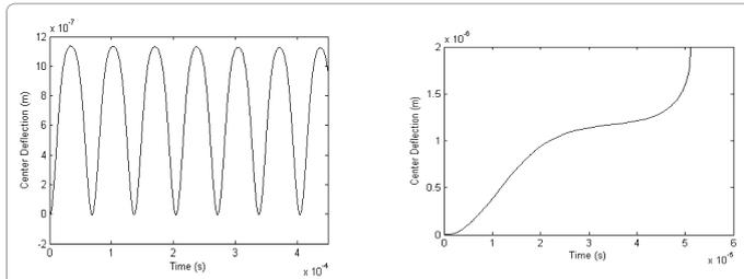
**Figure 22:** Dynamic response of the fixed-fixed micro-switch in the case of  $p=0$  subjected to step-wise DC voltage. (a) Time history of the micro-beam ( $V=9.61V$ ); (b) Time history of the micro-beam ( $V=9.62V$ ).
