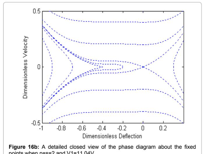
Figure 16b: A detailed closed view of the phase diagram about the fixed points when  $p=s=2$  and  $V_1=11.04V$ .
