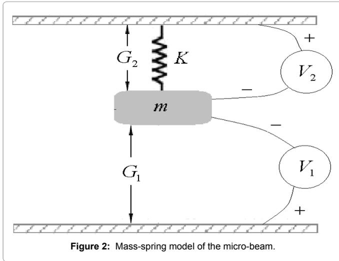
Figure 2: Mass-spring model of the micro-beam.
