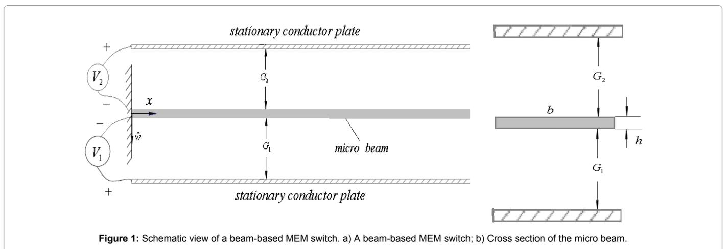
Figure 1: Schematic view of a beam-based MEM switch. a) A beam-based MEM switch; b) Cross section of the micro beam.
