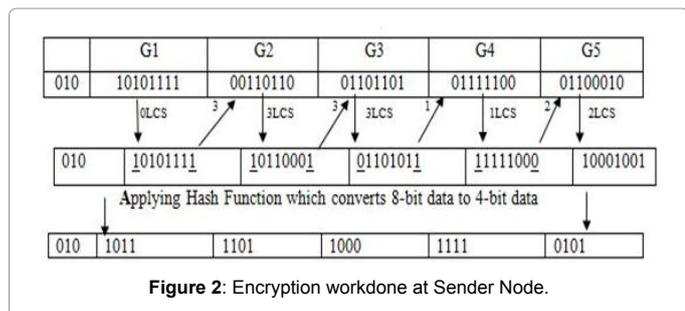
Figure 2: Encryption workdone at Sender Node.
