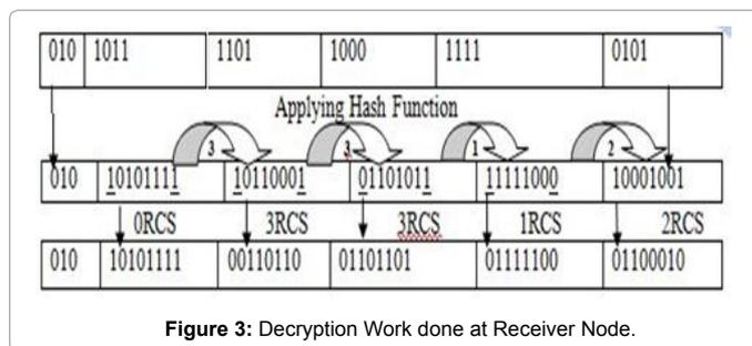
Figure 3: Decryption Work done at Receiver Node.
