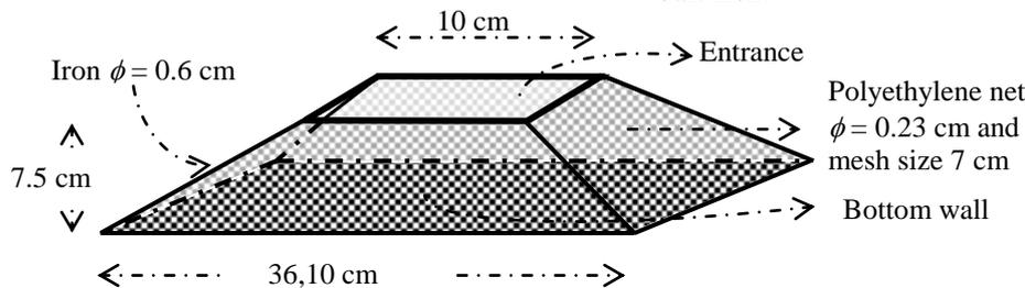
**Fig. 1.** Construction and dimension of "jodang" trap
