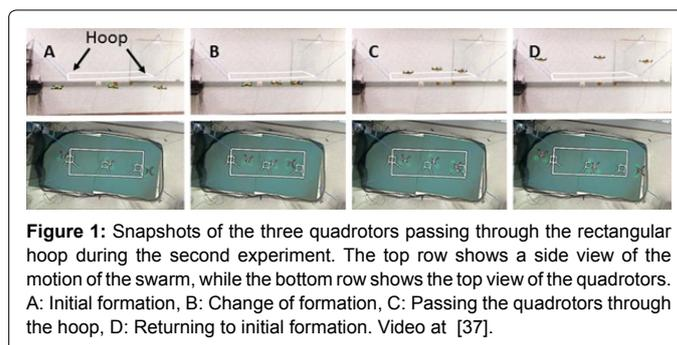
both the joystick and the brain interface to pass the swarm through the narrow hoop. This was a real-time demonstration of controlling a swarm of quad rotors using our proposed hybrid BMI using both EEG activations and joystick inputs.
