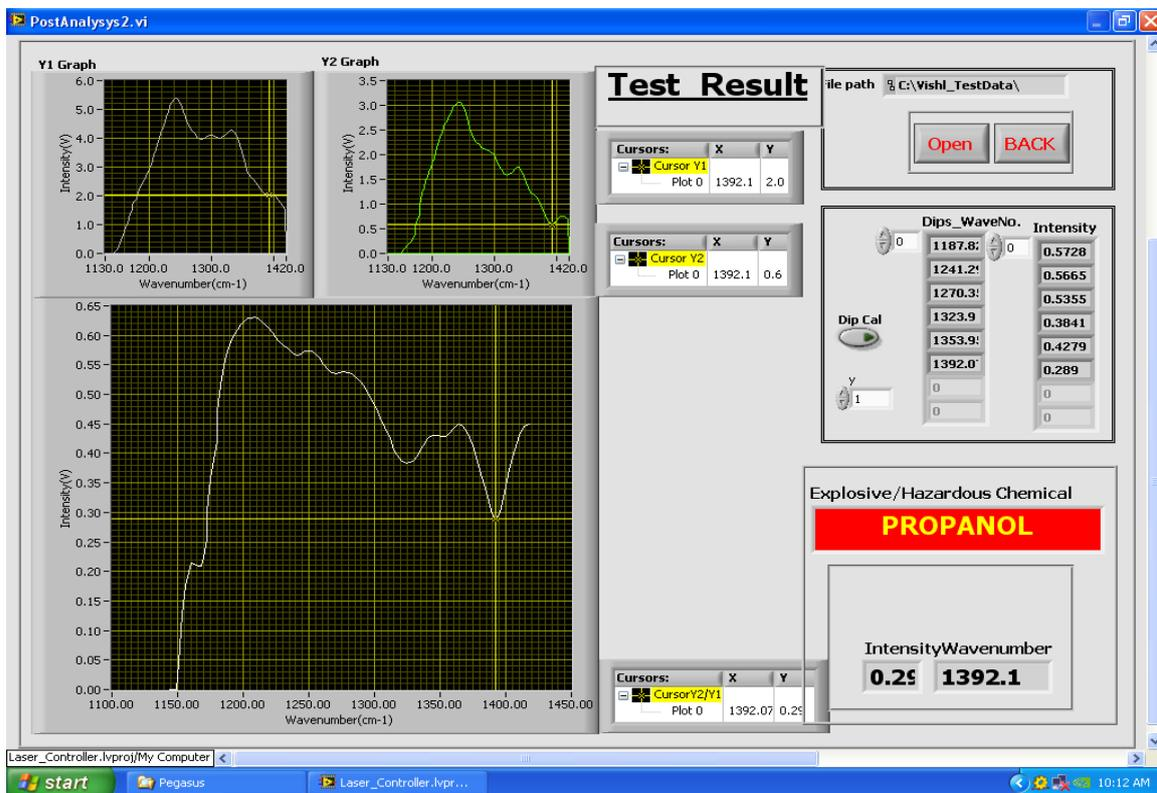
Figure 5e: Test Result GUI showing detection of propanol in liquid form from diffused aluminium surface.
