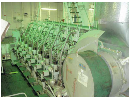
Figure 4: Main Engine on M/V JULES GARNIER (HITACHI MAN B&W 7S35MC Mk-7).
