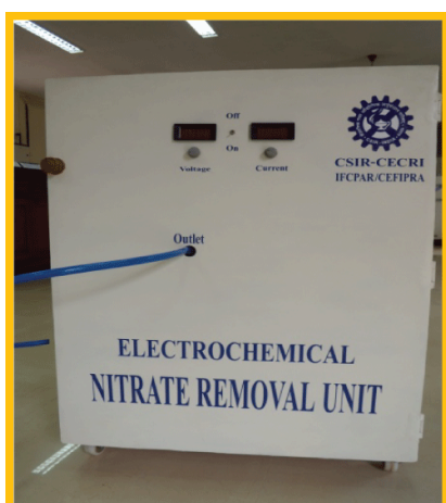
Figure 7: Electrochemical nitrate removal unit.
