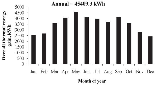
**Figure 2:** Monthly variations of overall thermal energy gain by combining a–d type weather conditions of a hybrid PVT array for Bangalore.
