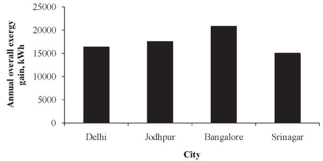
**Figure 5:** Annual overall exergy gain for four different cities of India by considering a–d type weather conditions of hybrid PVT array.
