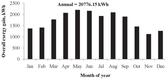
**Figure 3:** Monthly variations of overall exergy gain by combining a–d type weather conditions of a hybrid PVT array for Bangalore.
