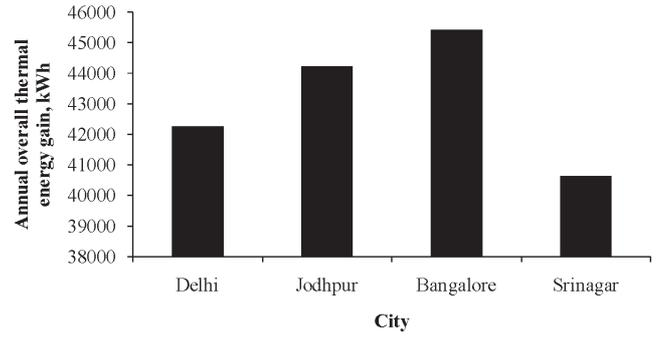
**Figure 4:** Annual overall thermal energy gain for four different cities of India by considering a–d type weather conditions of hybrid PVT array.
