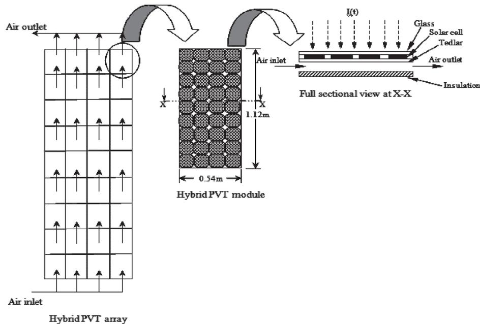
**Figure 1:** Typical layout of a hybrid PVT array showing flow configuration for case-I with an enlarged view of a PV module and its full sectional view (Rajoria et al. [10]).
