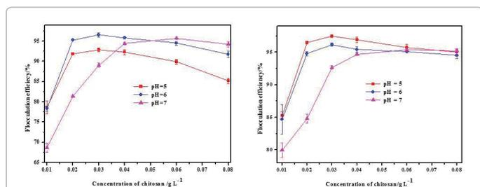
Figure 2: Effects of different pH on the flocculation efficiency of chitosan for biomass harvesting of tropic ocean oleaginous microalgae *Desmodesmus* sp. WC08 at the end of cultivation with different dosages at sedimentation time of 30 min (A) and 120 min (B), respectively.
