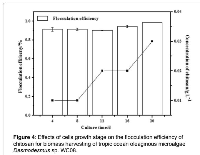
Figure 4: Effects of cells growth stage on the flocculation efficiency of chitosan for biomass harvesting of tropic ocean oleaginous microalgae *Desmodesmus* sp. WC08.
