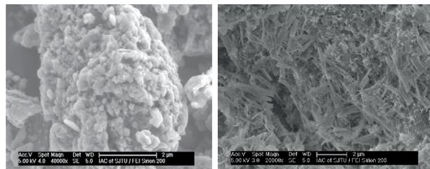
Figure 5: SEM Photographs of unsolidified ISSA and solidified block A. (a): unsolidified ISSA; (b): block A.
