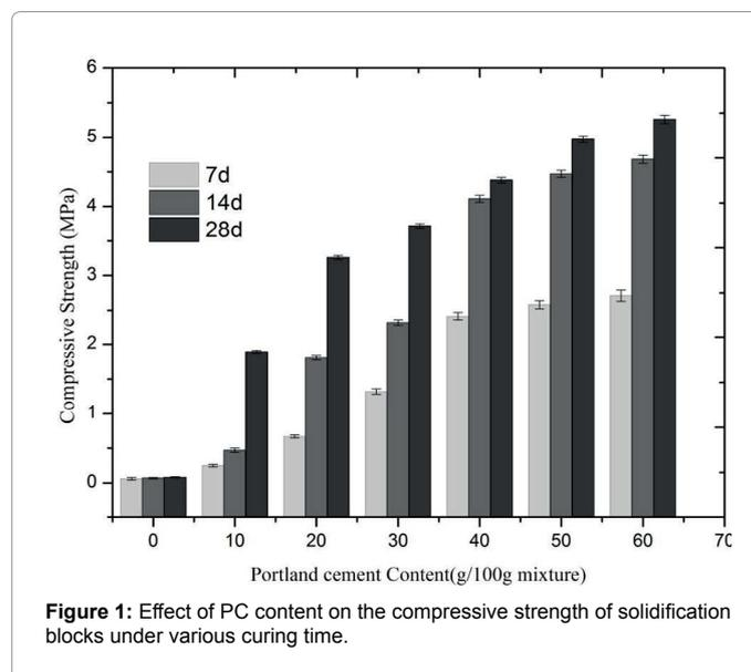
Figure 1: Effect of PC content on the compressive strength of solidification blocks under various curing time.
