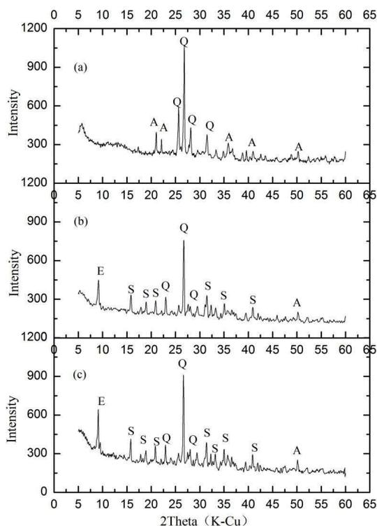
Figure 4: XRD patterns of three different samples. (a): untreated ISSA; (b): block A; (c): block B.
