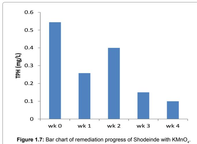
Figure 1.7: Bar chart of remediation progress of Shodeinde with KMnO<sub>4</sub>.
