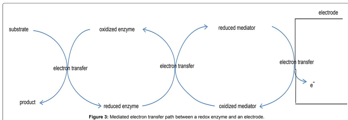
Figure 3: Mediated electron transfer path between a redox enzyme and an electrode.
