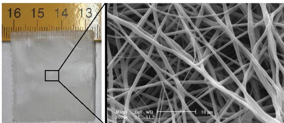
Figure 5: The fabricated hybrid bone scaffolds and its closed view.
