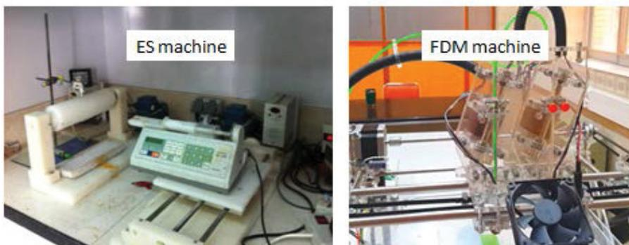
Figure 4: FDM and ES machines applied for fabrication of hybrid scaffolds.
