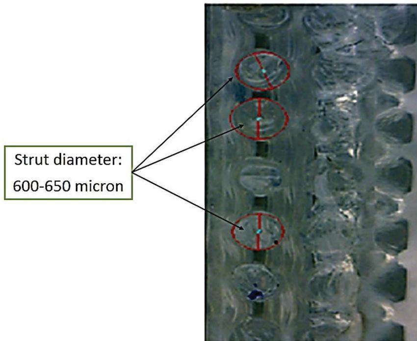
Figure 3: Side view of the pure fabricated bone scaffold fabricated by FDM technique.
