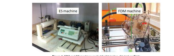
Figure 4: FDM and ES machines applied for fabrication of hybrid scaffolds.
