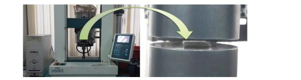
Figure 1: The front view of the compression test setup.
