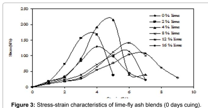
Figure 3: Stress-strain characteristics of lime-fly ash blends (0 days curing).
