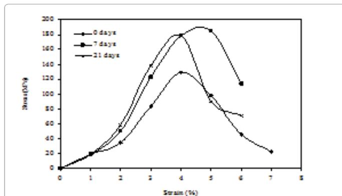
Figure 6: Stress-strain characteristics of lime-fly ash blends for different curing periods (0% lime).
