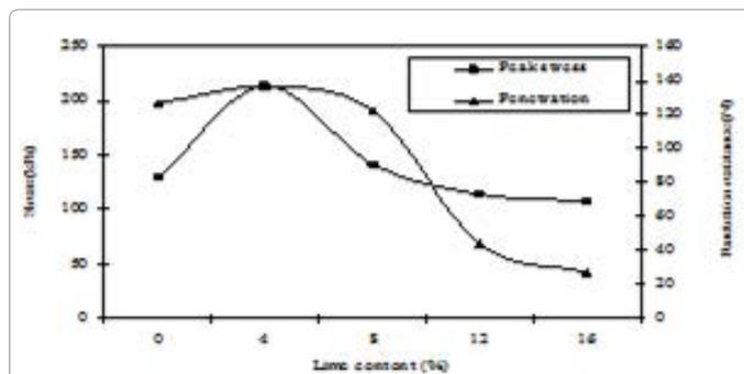
Figure 10: variation of peak stress and penetration resistance with lime content.
