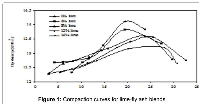
Figure 1: Compaction curves for lime-fly ash blends.
