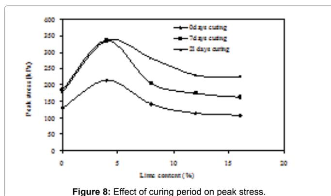
Figure 8: Effect of curing period on peak stress.
