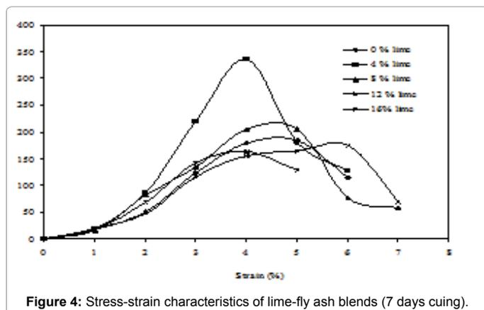
Figure 4: Stress-strain characteristics of lime-fly ash blends (7 days curing).
