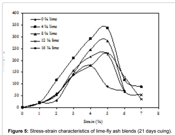
Figure 5: Stress-strain characteristics of lime-fly ash blends (21 days curing).
