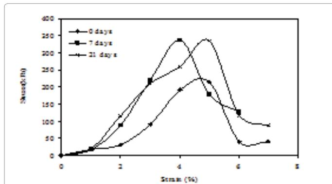
Figure 7: Stress-strain characteristics of lime-fly ash blends for different curing periods (4% lime).
