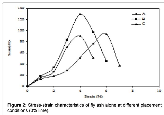
Figure 2: Stress-strain characteristics of fly ash alone at different placement conditions (0% lime).
