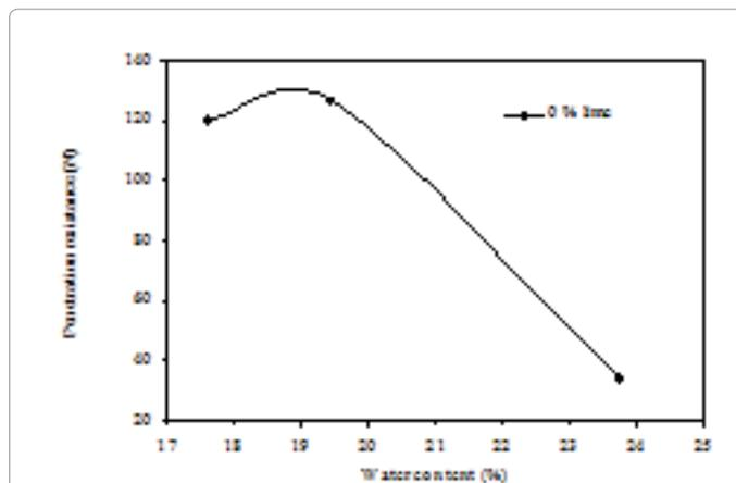
Figure 9: Effect of water content on penetration resistance of fly ash alone (0% lime).
